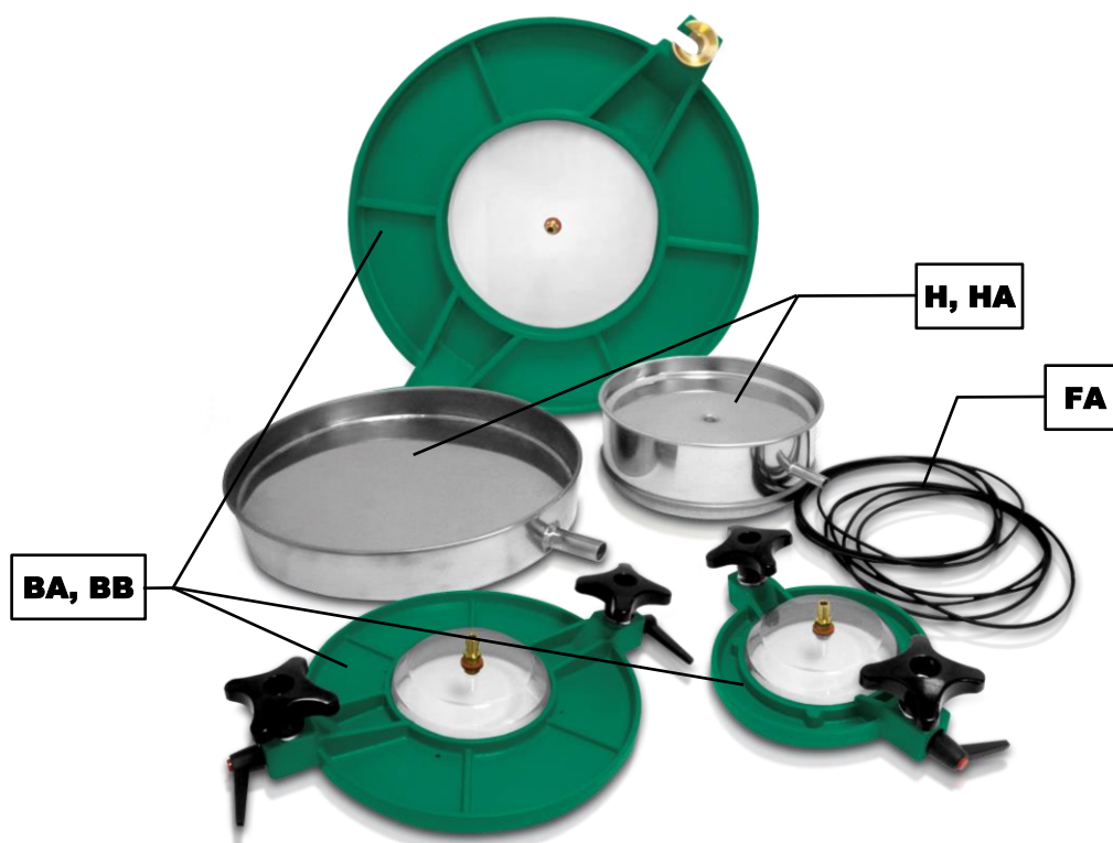
Fig. 11: Wet Sieving Adaptor Kit
